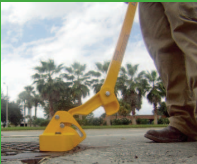
Place magnet on edge of cover
