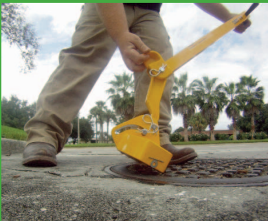
Push forward to release magnet
