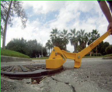
Push on handle to "break" seal
